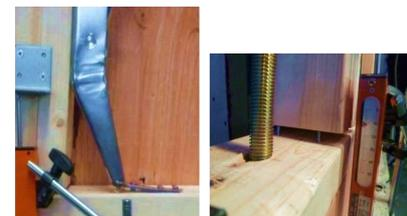
Figure 14: Ultimate state of test specimen
